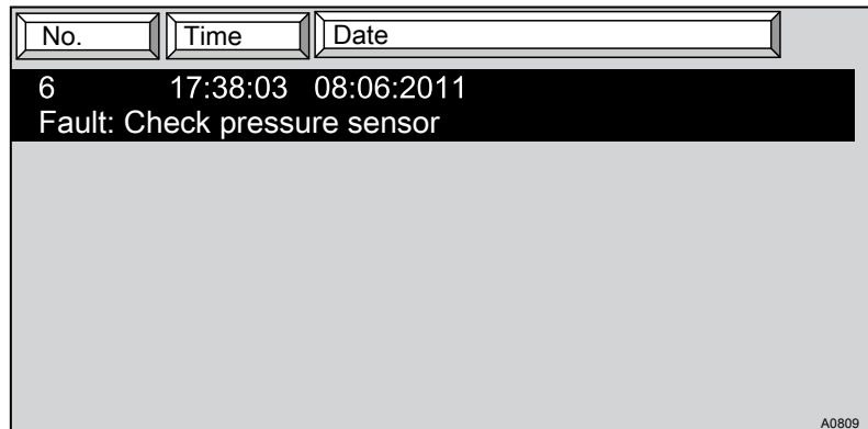
Fig. 53: Fault message on the display
